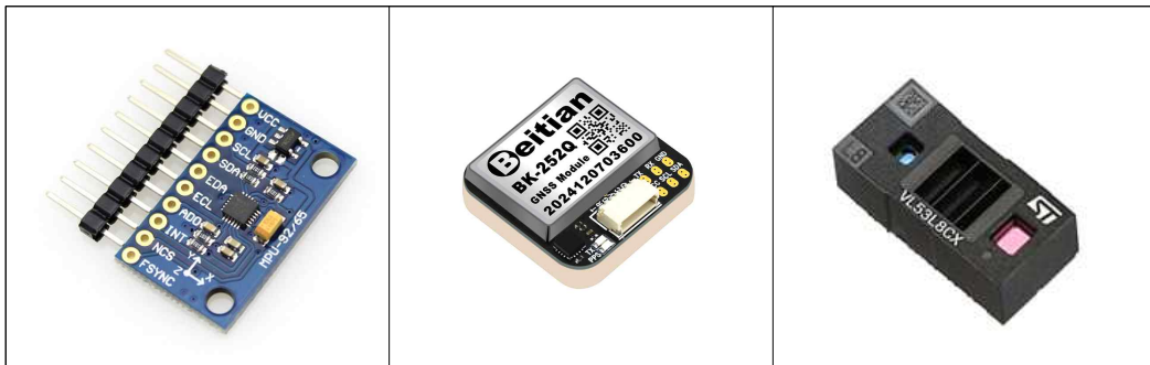
Fig. 15. MPU9250, BK-252Q, VL53L0X 센서
