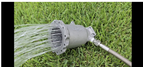
(a) Water-flow observation through the engine/injector article.
