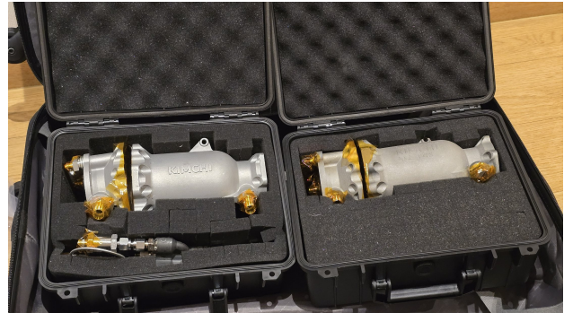
(b) Manufactured Kimchi Engine articles in protective cases before campaign integration.
